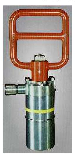
This unit known under its trade name of "Deep C" consists of twin magnetic sensing system complete with associated circuitry, in order to identify the passage of "Pathfinder" type of magnetic pigs or spheres.
