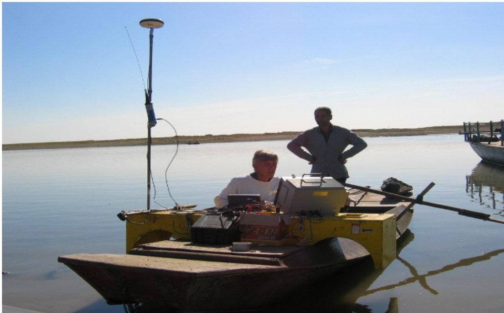
StarTrak personnel utilizing small fishing type boat in Northern China to conduct survey of 2500-ft river section
