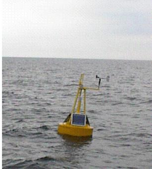
Passage alert is achieved by high intensity beacon on the surface buoy, also by means of Low Earth Orbit Satellite data communication link.
